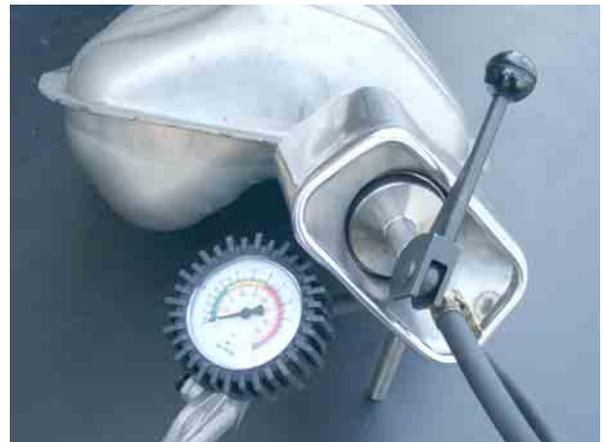
A sealing plug is fitted inside an exhaust and through the valve pressure is admitted to the system via a tyre inflator.
