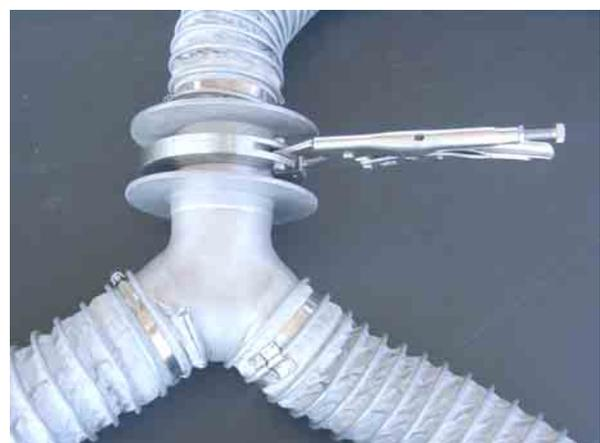
The pipe fittings are clamped to the Teflon hoses and large metal rings provide impact protection for the flange.
