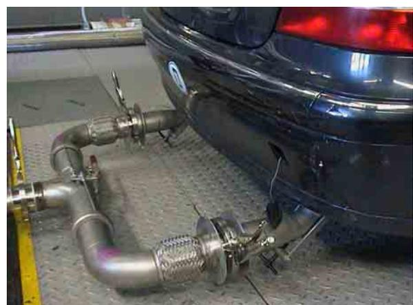
For cars with a double-flow exhaust system the Bleyer staff designed these "antlers", which have a variable width.
