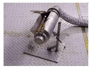
The collecting funnel is placed at the exhaust when a vehicle is being conditioned in order to extract the exhaust gases.
