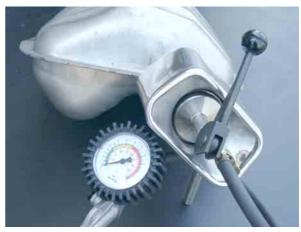
A sealing plug is fitted inside an exhaust and through the valve pressure is admitted to the system via a tyre inflator.
