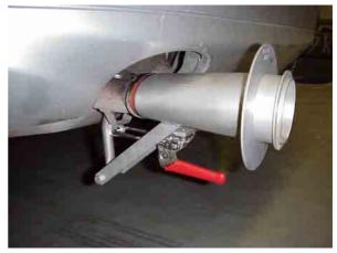
The exhaust gas removal adapter is attached to the exhaust pipe with the red lever, making a gas-tight connection.
