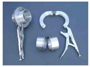
The closed locking pliers (left) hold two pipe fittings together. The open pliers and pipe fittings are on the right.
