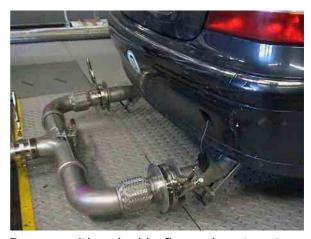
For cars with a double-flow exhaust system the Bleyer staff designed these "antlers", which have a variable width.
