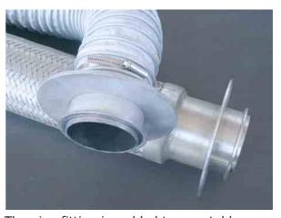
The pipe fitting is welded to a metal hose or clamped to a Teflon hose with a clip. Both connections are gas-tight.
