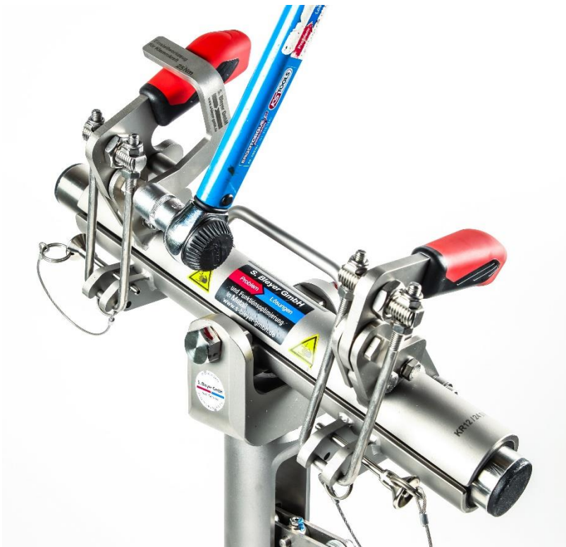
Figure 34: Adjusting tool for setting the clamping force
