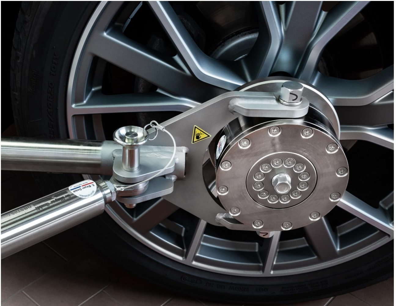
Figure 31: Correctly mounted ball lock pin
