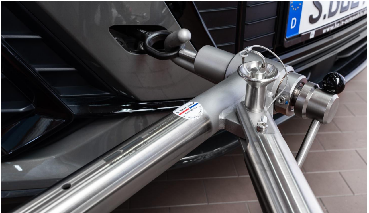
Figure 27: Correctly mounted ball lock pin
